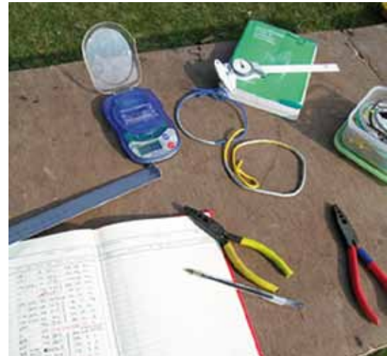
Figure 2.33. A typical ringing kit, showing ringing pliers, rings, weighing balance, wing rule, callipers and, perhaps most importantly, a notebook and pen! (photo: BTO).
