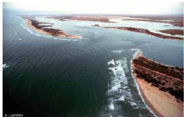
Figure 5.5. The breach in the Langue de Barbarie (Barbary spit) made as a small opening in 2003, now clearly an established wide channel; beforehand the spit was continuous, separating the Senegal River from the Atlantic Ocean (photo: L. Gerrler).
