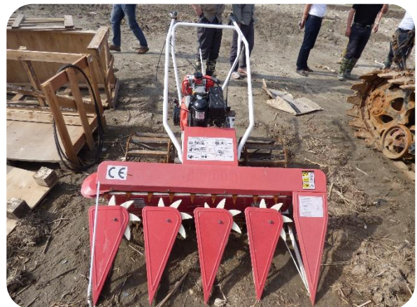
Different machines can be used to cut Spartina . Pictured here is a mini harvester/cutting machine. [Credit: David Melville].
