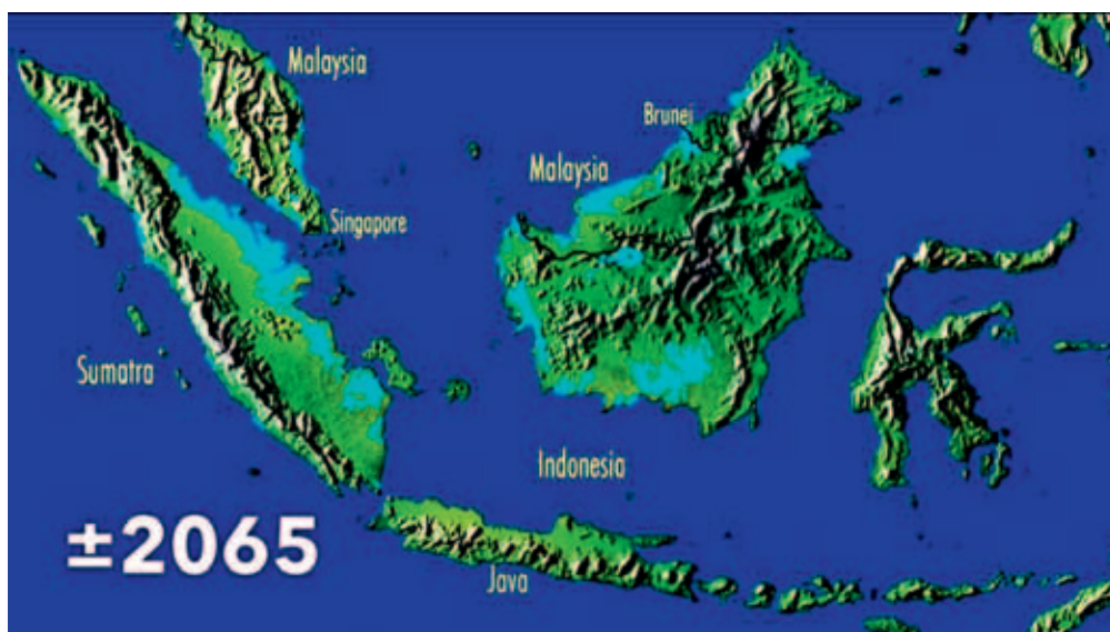
Figure 2. In Southeast Asia, extensive low-lying areas (light-blue) are degrading and experiencing soil subsidence as a result of deforestation and drainage. Many of these are expected to become unproductive as a result of frequent and prolonged flooding, affecting the lives and livelihoods of local communities and resulting in large economic losses.
