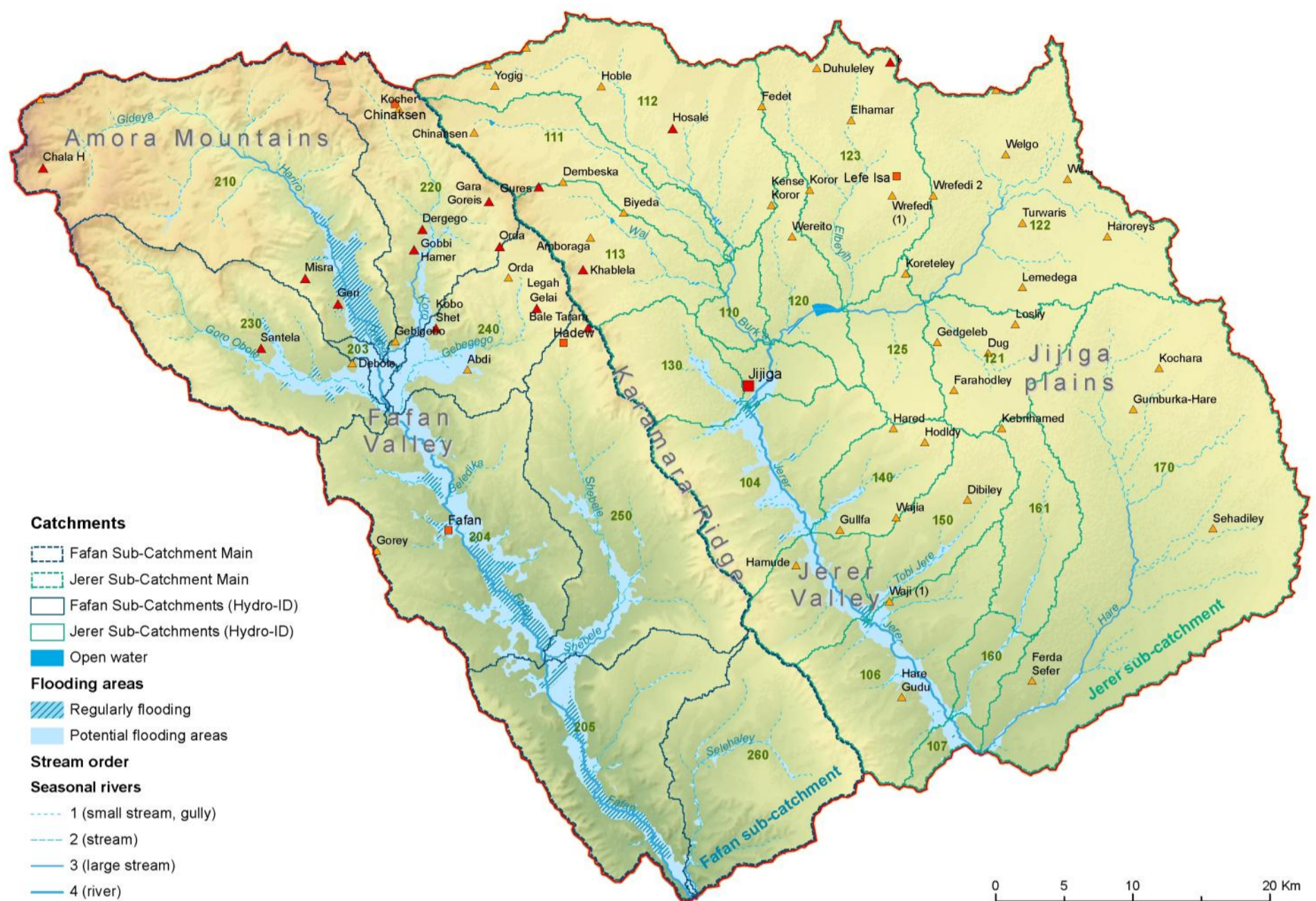
Figure 4.4 Surface water bodies, flooding areas and Hydro-ID used for rainfall-runoff calculations. For both Fafan and Jerer Rivers applies that floodplains and wetlands play an essential role in regulating flows and supplying groundwater for agriculture and domestic use.
