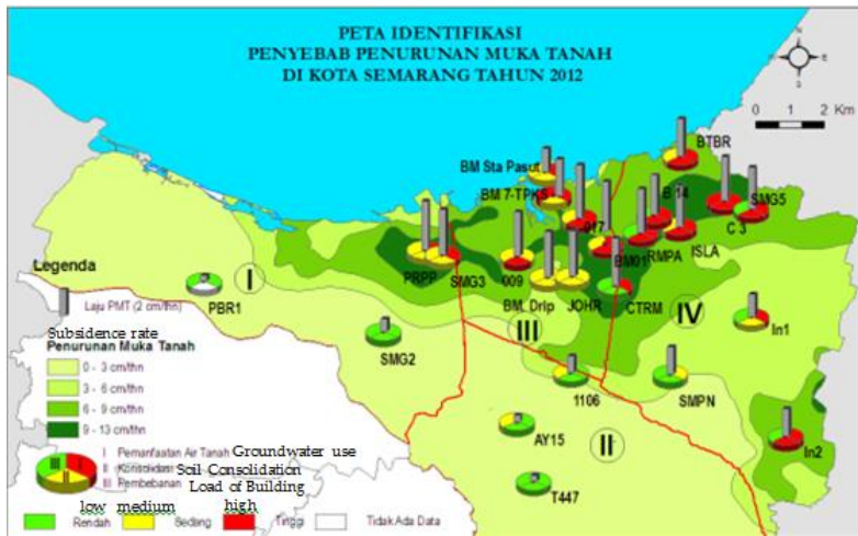
Figure 2.9 Land subsidence causes indication in Semarang (Yuwono, 2013)
