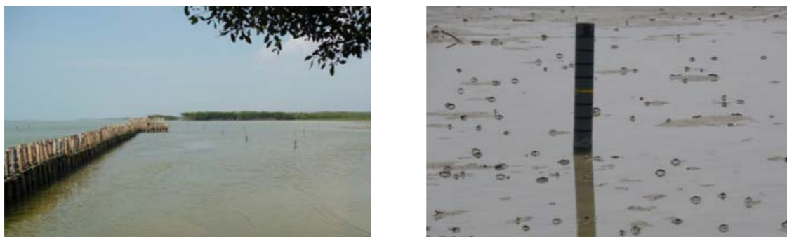
Figure 23. Monitoring sedimentation with sedimentation poles © Tom Wilms, Witteveen+Bos
