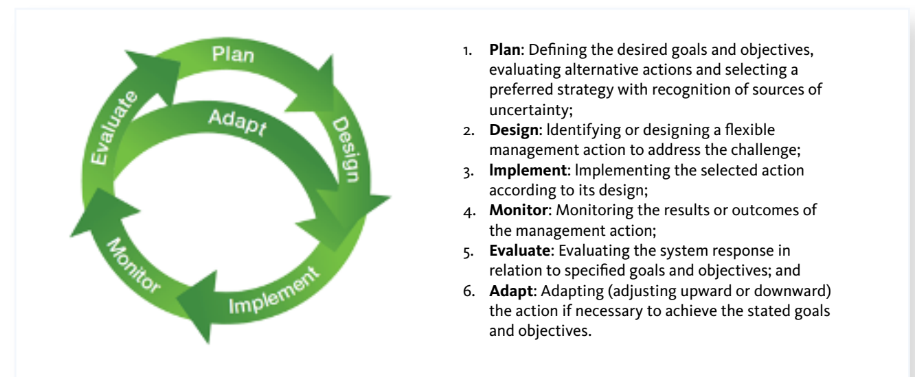
Figure 3.3 Adaptive monitoring and maintenance cycle (CEDA, 2015) based on (Fischenich and Vogt, 2012).
