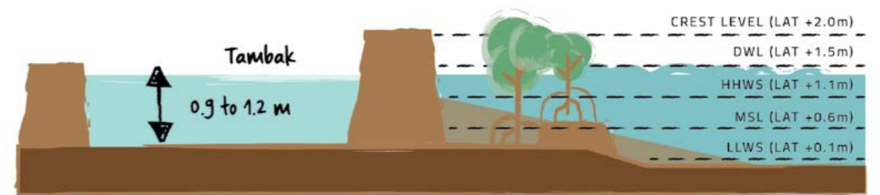
Figure 13f: After the new dyke is constructed and the pond is filled with water, the old dyke can be adapted as a mangrove habitat, with moderate amount of fill material needed. The new habitat starts at HHWS, with length of minimum 10 m.
