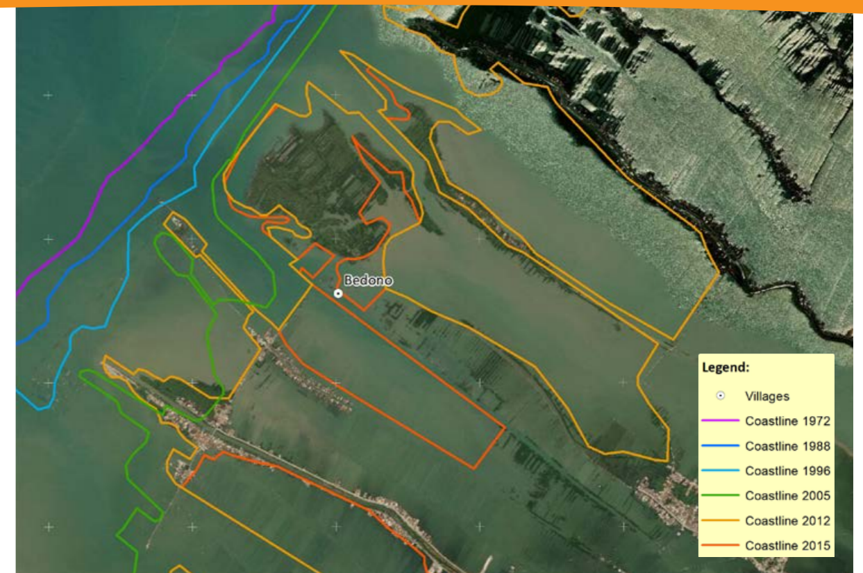
Figure 1. Coastline changes Demak (north-east of Semarang), 1972-2015 (© Wetlands International, based on maps from Aerial photography, WorldView, Landsat, US Army, Peta Rupi Bumi Indonesia).
