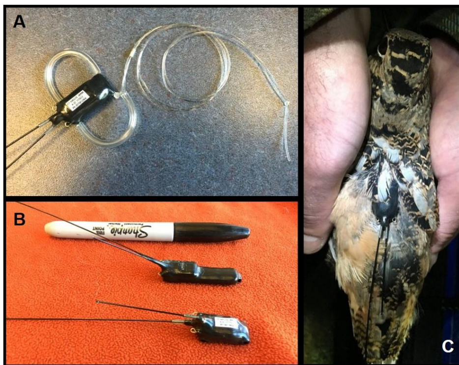
Figure 1. Examples of A) transmitter leg loop harness, B) 6.3 g (top) and 4 g (bottom) GPS transmitters with standard sharpie marker for scale, and C) positioning of transmitter on the back/rump of a marked American woodcock.
